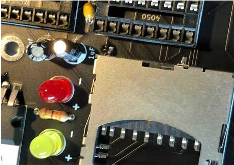
If you are satisfied with the lineout solder the other 3 outside clips of the holder to the PCB. After this solder the inside contacts and try to use not to much solder on the contacts because otherwise the SD card cannot be entered. If you have soldered all the contacts take a magnifying glass to check if all the contacts make a good connection and make no contact with each other due to solderbridges.
