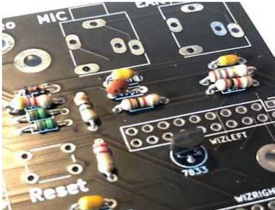
Place the flat side of the two 78133 exactly the same as indicated on the pcb.
