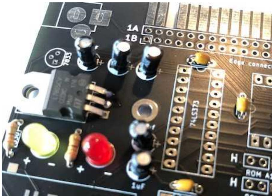
Now we are placing the voltage regulators 7805 and the two 78L33. Do look carefully at the codes on the 78L33. They look the same as the transistor BC547, **SO DO NOT MIX THEM UP!**
