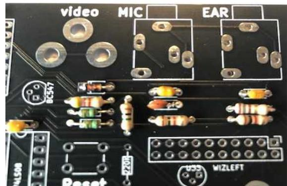
Resistors have no polarity so can be placed on the PCB as you like.. After you have placed all the resistors you can put the two LEDs in place. LEDs do have a polarity. So look carefully at the picture. The long leg of the LED goes in the + indicator.
